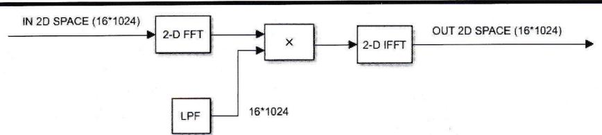
**Figure 10 — Block diagram of the low-pass filtering in space.**
